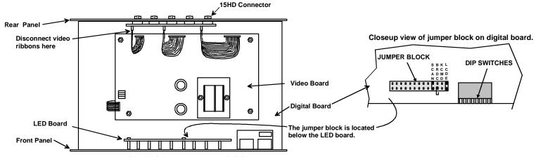
Overhead view of video board on top of digital board.
